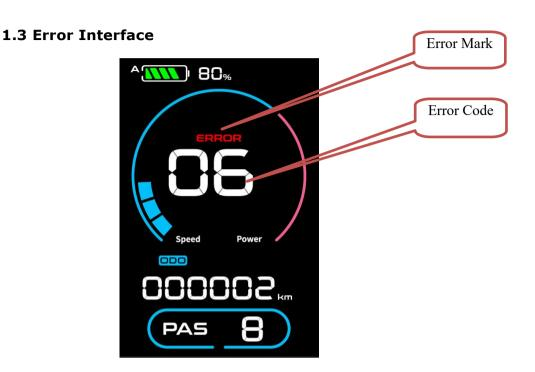
In the above interface: Error Indicator: ERROR, Error Code: 06
